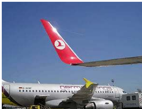
Boeing's 737 wingtips in the foreground in red are clearly different from those on the Airbus 319 (in yellow).
